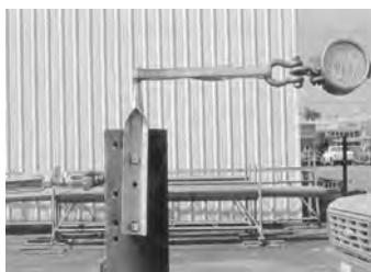
1500 lbs. transverse load with no deformation, 2770-A20-100.
