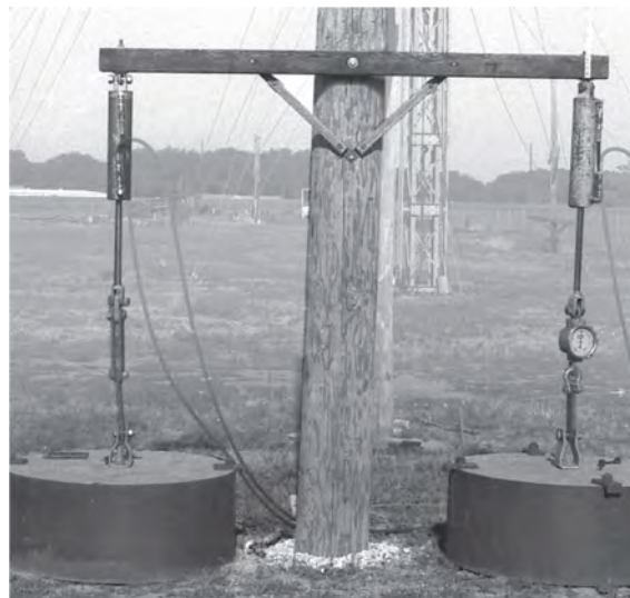
Pair of 2023 braces removed after 20 years of service ready for testing. These braces performed to full capacity when tested.
