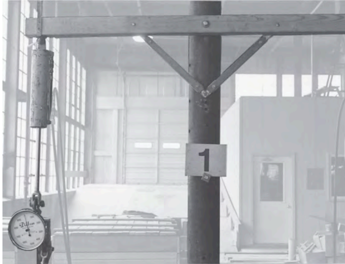
2023 Brace ready for testing in accordance with REA specs.
