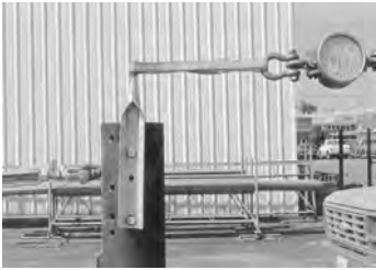
1500 lbs. transverse load with no deformation, 2770-A20-100.
