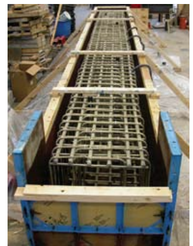
Full scale D-wall unit strip testing, University of Missouri Rolla.
