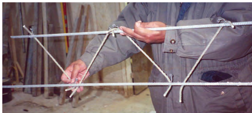
Fig. 3. Fiber reinforced shear connector.
