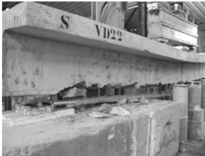
Fig. 6 Peeling off of the GFRP strengthening - Beam D.2
