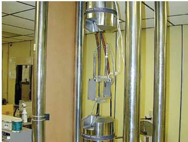
Aslan 500 CFRP tape being tested
