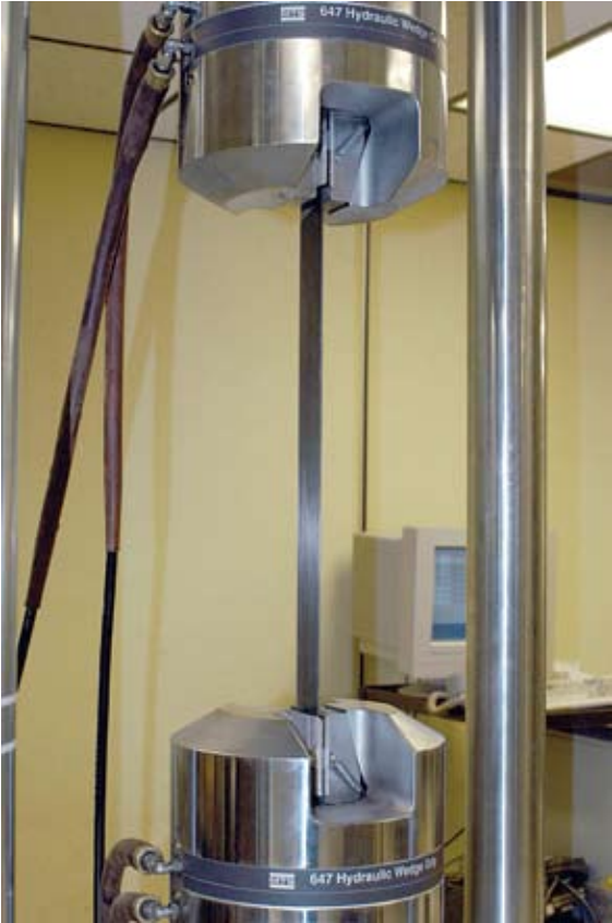
Aslan 400 CFRP Laminate testing
