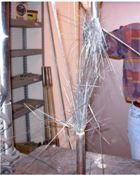
Figure – 6. Brooming failure of CFRP bars assembly.
