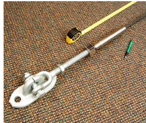
Figure – 4. Photograph of dead-end of CFRP bar assembly.
