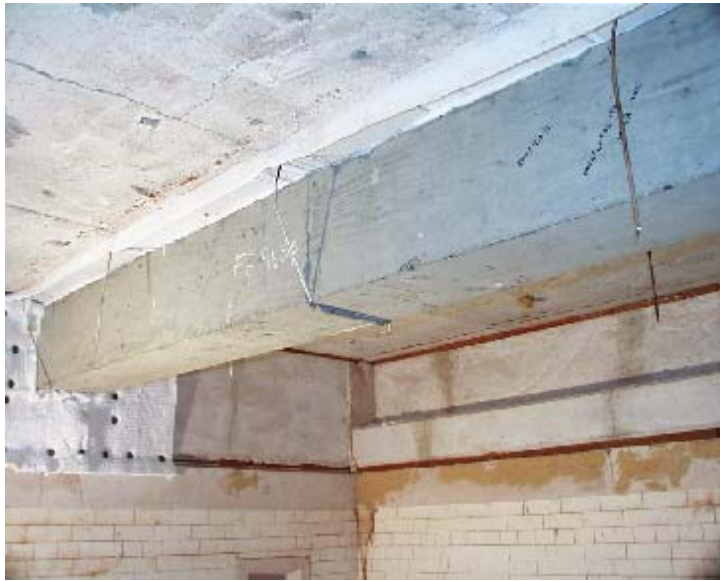
Fig 3c Beam is set inside the insulated furnace for fire test
