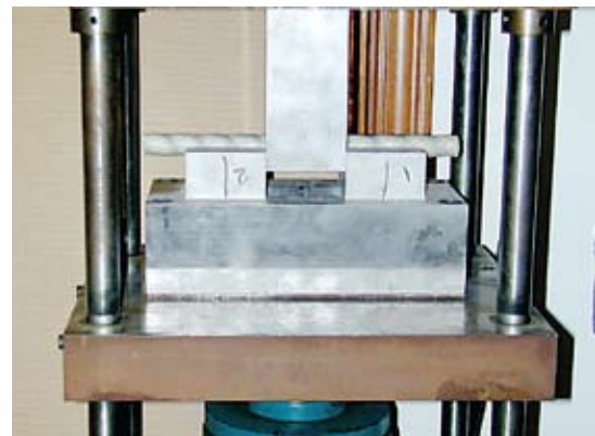
Shear Strength Test Fixture
