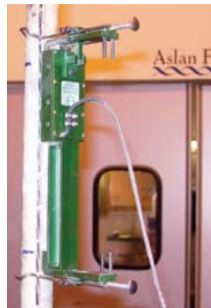
Extensometer measuring elongation during tensile test.
